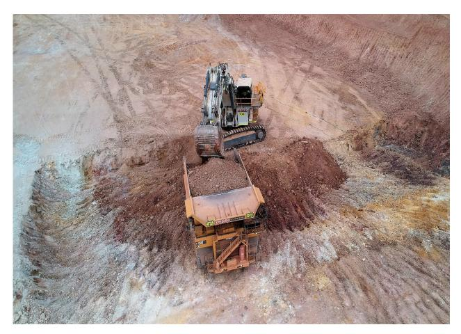
Figure 8 – 200t excavator at work in the Riverina Open Pit
